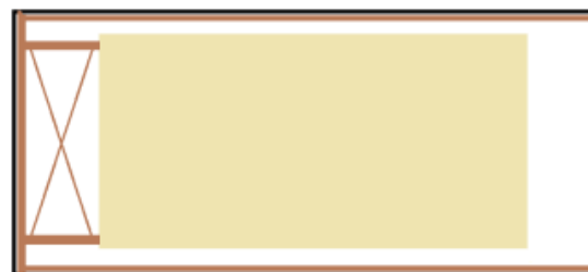
Bulkhead with compression members
